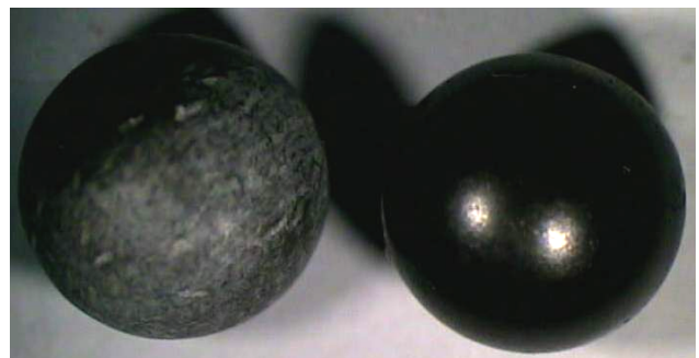
\text{Si}_3\text{N}_4 – Ball before and after grinding
