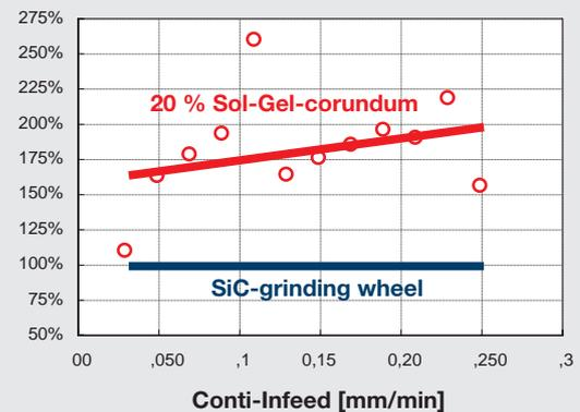
**Diagram 1:** Comparison of the specific machining performance [ $\text{cm}^3/\text{min}/\text{kW}$ ]
