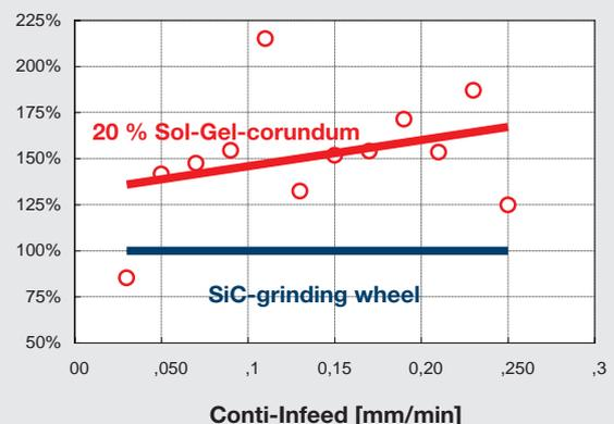
**Diagram 2:** Comparison of the G-ratio [ $\text{cm}^3/\text{cm}^3$ ]
